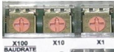
Figure 11 – Address Selection Switches
