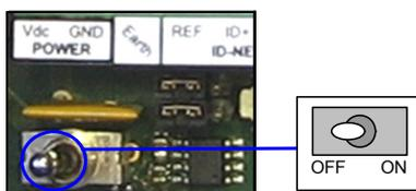
Figure 14 - Power Switch ON/OFF Positions
